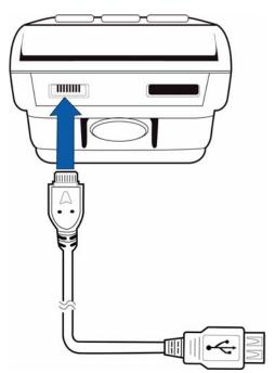
Figure 5 **USB Host Cable Connection to a V<sup>x</sup>670 Terminal**
